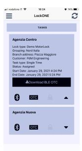
Before to reach the safe, user download OTC data with his smartphone app from the web server. Data can be downloaded for a single task within the assigned ones or for all assigned tasks.
