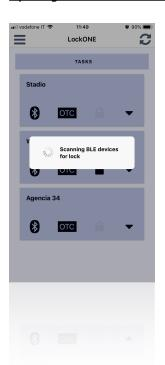
Once in front of the safe, user starts Bluetooth mode on the lock keypad by entering a valid 6-digit code and then clicks on selected task Bluetooth button on his smartphone app. Once communication between smartphone and lock is established and authorization to open is confirmed, user will be asked to enter is personal identification number (PIN) into the LockOne app
